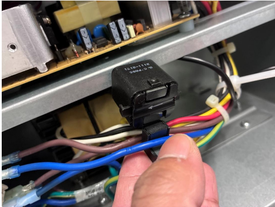
Figure 27 – CT Clamp Installation Example
