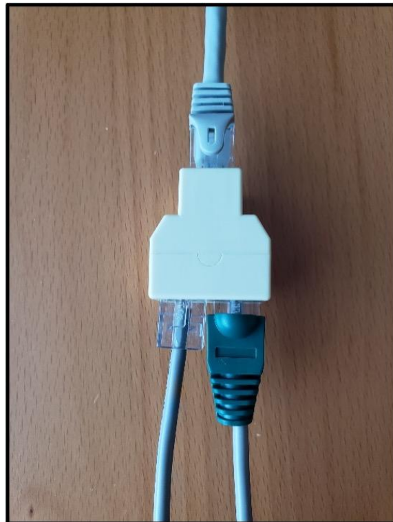
Double-door sensor switch connection to dongle
