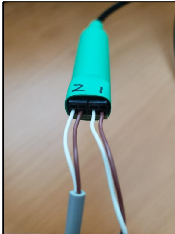
Two door switches connected to a SmartCable-DI
