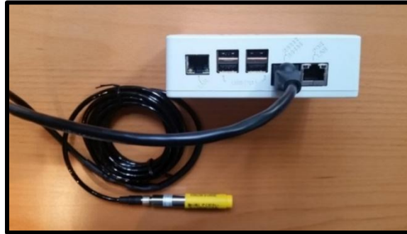
Sensor connected to RS232/RS485 port
