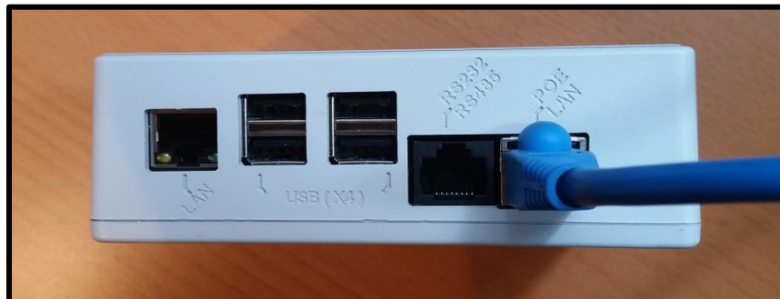
Ethernet cable connected to PoE/LAN port from PoE injector, PoE switch, or PoE-enabled outlet
